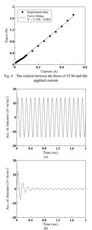
Fig. 5 Response of the anti-vibration under an excitation at 8 Hz, (a) without control, (b) with control
