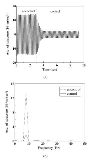
Fig. 7 Response of the anti-vibration under an excitation at 8Hz, (a) time domain; (b) frequency domain.
