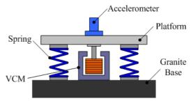
Fig. 3 The setup of the active vibration isolation system
