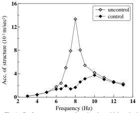
Fig 6 Performance test result under sinusoidal excitation.
